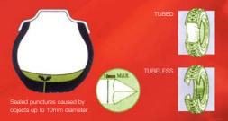
puncture. When the puncture occurs, the escaping air pressure forces Linseal into the hole immediately forming a strong airtight seal.
