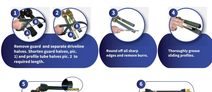
Reassemble guard halves. Both profile tubes should extend 40-mm (1.58") beyond the end of the guard tubes.
