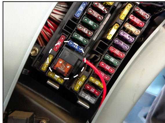
Fig. 48: Connect the connection cable with the blade-type fuse adapter
