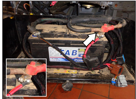
Fig. 59: Power connection to vehicle battery
