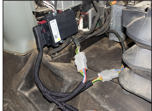
Fig. 50: Connecting the ISOBUS TECU adapter to the main harness and the vehicle
