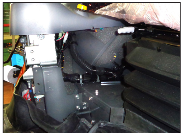
Fig. 23: Lining from side console removed
