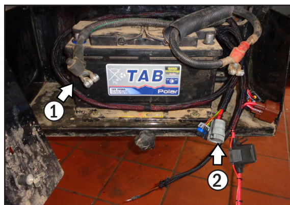
Fig. 37: Lay excess cable in loops
