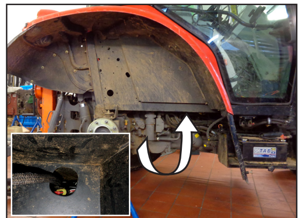
Fig. 33: Cable lead-in into the cabin
