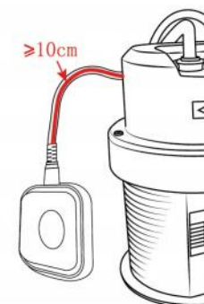
Cable more than 10cm
