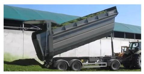
For example in tippers with single large cylinders, the return stroke can cause sudden flow surge, lasting for a few moments, potentially damaging the seals of the hydraulic couplings.
