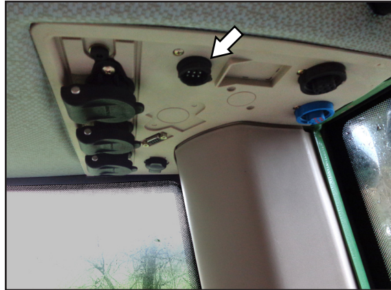
Fig. 13: Connect Joystick in cabin
